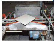
and the PU construction lasted more than five times longer than the previous grip tops.
