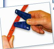
belt off, take out a link and roll it back on — no need to move any drive components.
