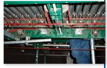
installed, PowerTwist Roller Drive lasted three times longer than a rubber belt on their most problematic conveyor.
