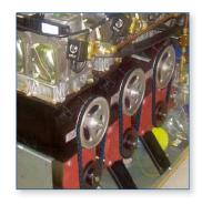
able to tap into all the benefits of a Fenner Drives HPC V-Belt while providing a safe and reliable solution. Belt life on the pumps was increased and service technicians always have the correct belt on hand in these remote locations.
