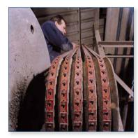
Solution Installing NuTLink V-Belts reduced downtime to just two hours with the added bonus of longer belt life.
